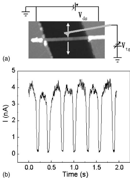
FIG. 3. (a) A schematic of scanning tip gating, a negatively biased conductive tip is scanned across the nanowire; (b) time domain measurement of scanning tip gating. Nanowire conductance is modulated periodically.
