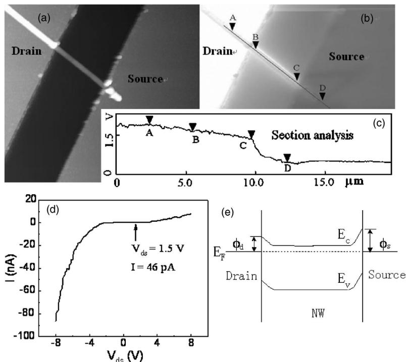
FIG. 1. (a) Topography image and (b) surface potential image of a ZnO nanowire FET with Ni electrodes. (c) Section analysis of the potential profile along the nanowire channel. (d)  $I$ - $V$  characteristic from electrical transport measurement. (e) Energy band diagram illustrates the asymmetric Schottky barriers at the source and the drain contacts.
