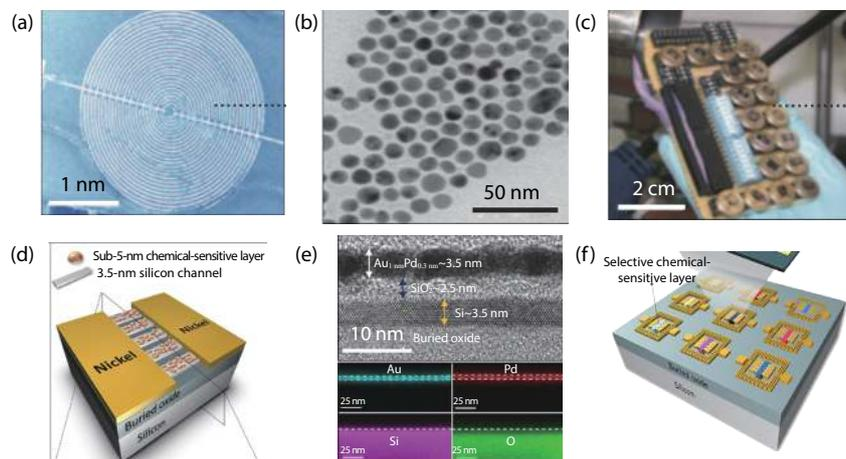
Fig. 3. (Color online) (a) Sensor array fabrication methods and morphology<sup>[12, 13]</sup>: (a) an SEM image of organic functionalized gold nanoparticle film deposited between adjacent electrodes, (b) a TEM image of monolayer capped gold nanoparticles, (d) a TEM image of ultrathin silicon channel, (e) EDS indicating the elemental composition of a single Pd-Au CS-FET, gas sensor array of (c) gold nanoparticles, (f) CS-FET.
