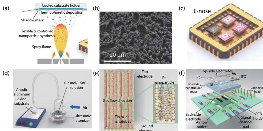
Fig. 2. (Color online) MOX sensor array fabrication method and morphology<sup>[10, 11]</sup>: (a) FSP set-up, (b) SEM image of porous doped SnO<sub>2</sub> film, (d) USP setup, (e) Cross-section of SnO<sub>2</sub> nanotube decorated with Pt nanoparticles, gas sensor array of (c) doped SnO<sub>2</sub> microsensors and (f) 3-D SnO<sub>2</sub> nanotube.
